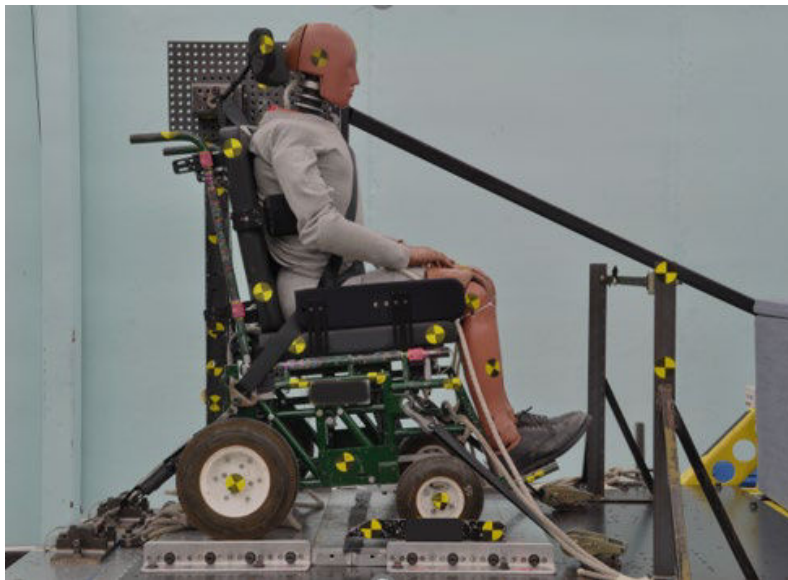
Figure 7 – Manufacturer's seating system installed on the surrogate wheelchair frame (SWCF) secured facing forward on the UMTRI sled by the surrogate four-point, strap-type tiedown and loaded with a Hybrid-III midsize-male ATD
