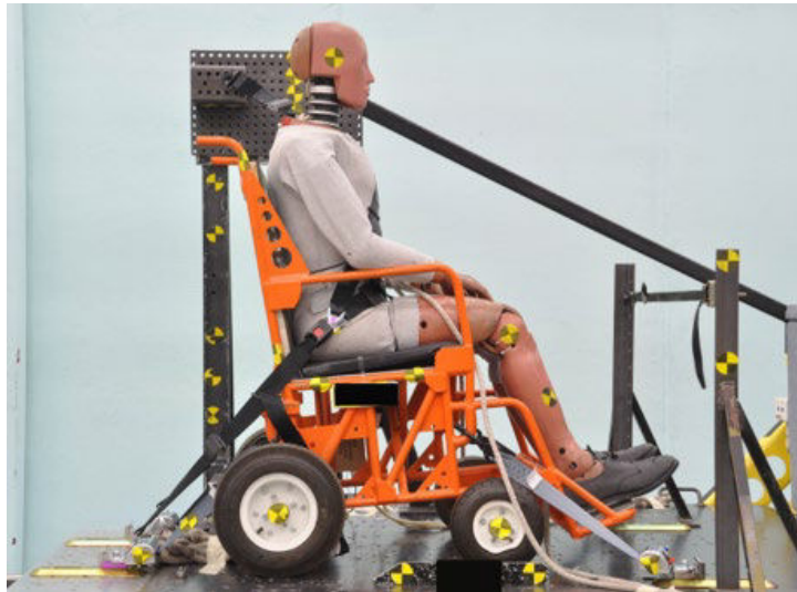
Figure 6 – 187-lb surrogate wheelchair (SWC) loaded with the Hybrid III midsize-male ATD restrained by a commercial lap/shoulder-belt restraint and secured facing forward on the UMTRI sled by the WTORS manufacturer's strap-type tiedown system
