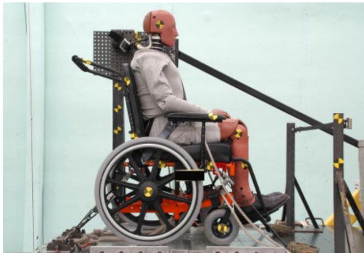
Figure 5 – Wheelchair secured facing forward on the UMTRI sled using the surrogate four-point, strap-type tiedown
