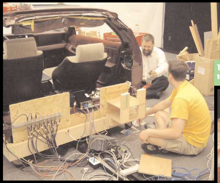
Inputs and outputs to the new video system in the buck are installed.
